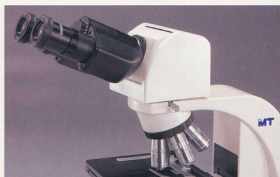
MA957 ERGONOMIC TILTING BINOCULAR HEAD (SIEDENTOPF TYPE)
