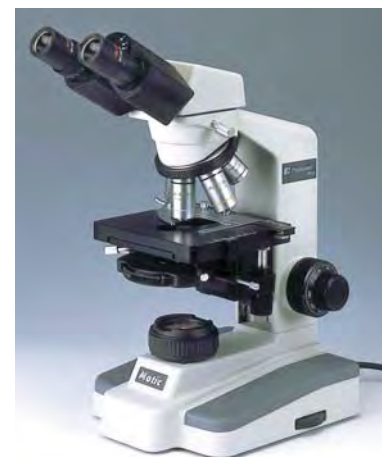
B3 with phase contrast attachment
